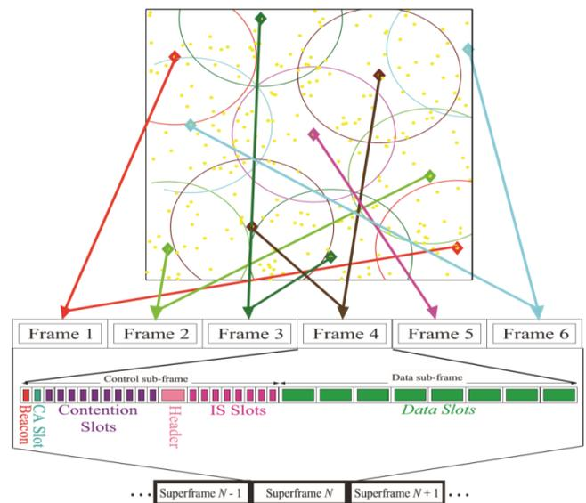
Fig 1: A snapshot of MH-TRACE clustering and medium access.
