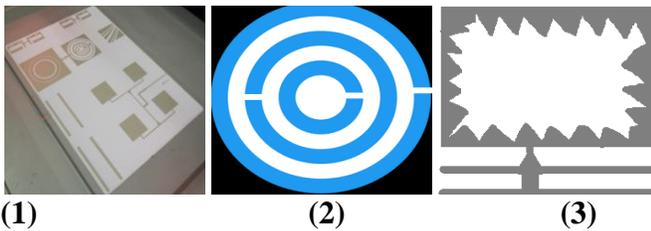
**Figure 2 (1)Feed line printed antenna on paper (2) Split ring resonator (3) Fractal stacked patch antenna**
